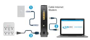
1. Connect the coaxial cable from the wall outlet to the coaxial connector on the back of the modem (hand-tighten to avoid damaging connectors). Contact Sunwire if you cannot find the wall outlet.
